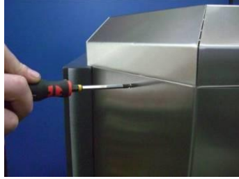
Figure 03: Replacing heating elements
